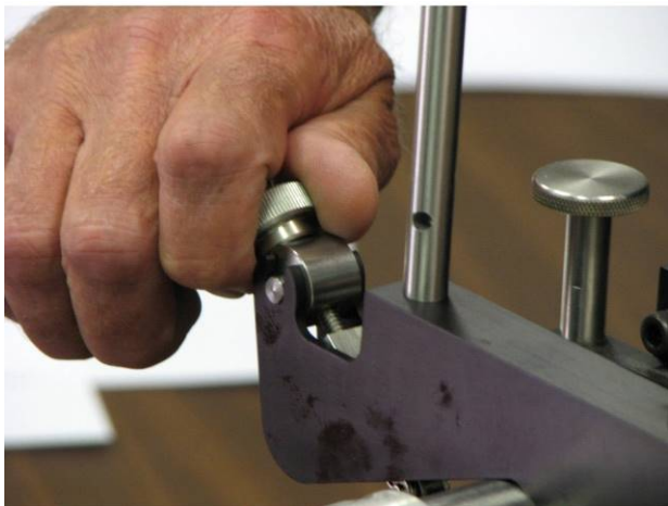
Tighten knob and fold chain (see 2B and 2C on Page 21)
