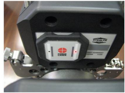
Figure 45 -- Aligning laser beams with S-670 to take uncoupled shaft data in Point Mode using the dust cover/alignment tool.
