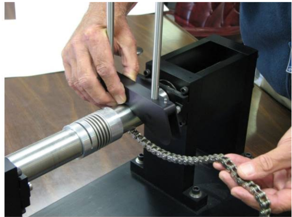
Wrap chain around the shaft
