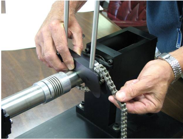
Attach chain to pin on A-970 bracket
