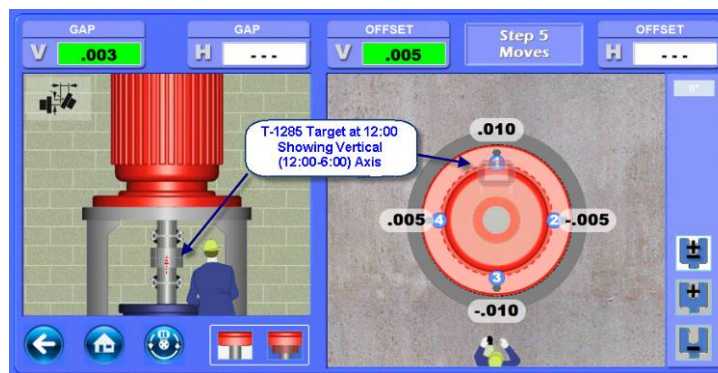
Figure 65 – Step 5: Vertical Pump Move Screen using the T-1285 Target at 12:00, showing Vertical Axis
