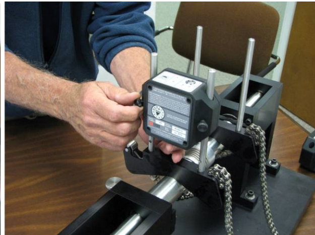
Slide target on A-970 bracket
