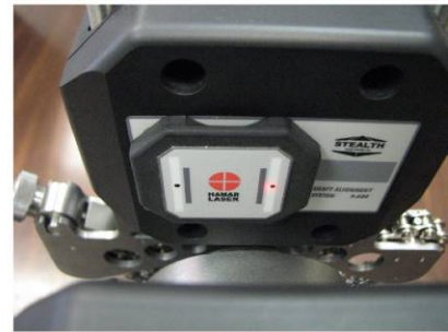
Figure 52 -- Aligning laser beams with S-670 to take Uncoupled Shaft data in Point Mode using the dust cover/alignment tool.
