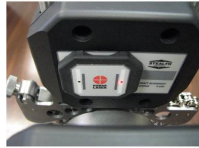
Figure 30 – Laser beams not aligned (left); Laser beams aligned (right)
