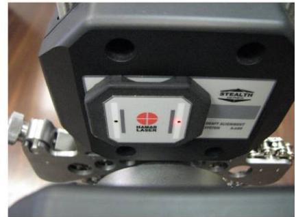
Figure 55 -- Aligning laser beams with S-670 to take Uncoupled Shaft data in Point Mode using the dust cover/alignment tool
