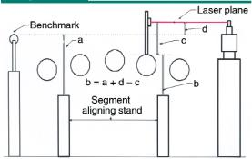
The vertical distance from the laser plane is measured for each roll using the height gauge target. Software calculates the shimming required to reach specification. Legend: a = distance from aligning stand pad to benchmark; b = alignment specification; c = measured distance from roll surface to laser plane; d = measured distance from bench mark to laser plane.
