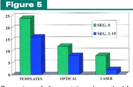
Comparison of alignment times by method for No. 1 caster.
