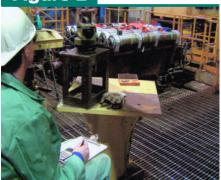
The second generation alignment method employed use of an optical level. This method cut alignment time approximately in half, but variability was still an issue.
