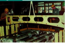
Originally segment rolls were aligned using templates and feeler gauges, introducing significant variability.
