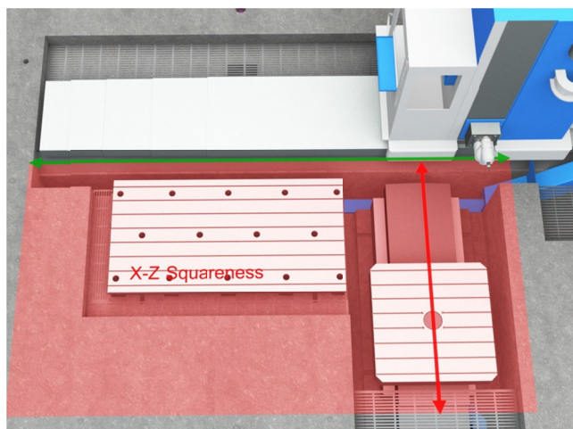
Horizontal Floor Mill with 30 ft X Travel and 5 ft Z Travel
