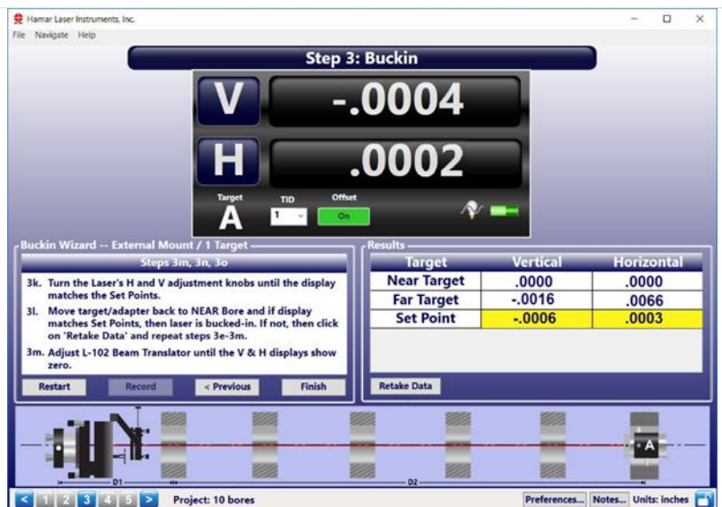
Bore9 - Step 3: Laser Steered to Near Zero (Bucked-In to within .0001 in.)
