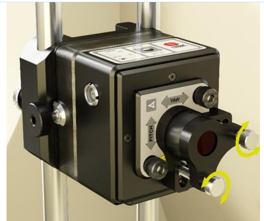
L-103 Laser Beam Translator Adjustments
