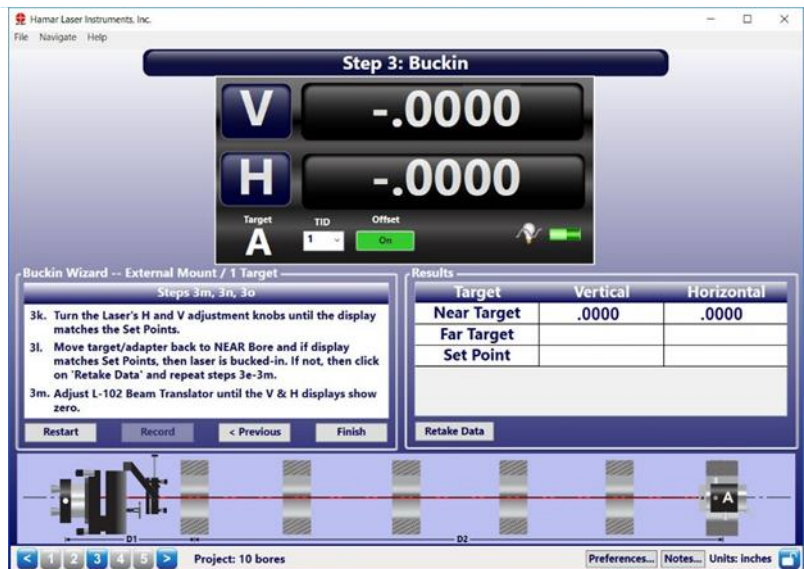
Bore9 - Step 3: Data Taken Near Bore
