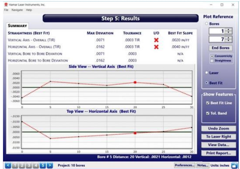
Bore9 – Step 5: Results – Straightness Plot using the Best Fit line as a reference
