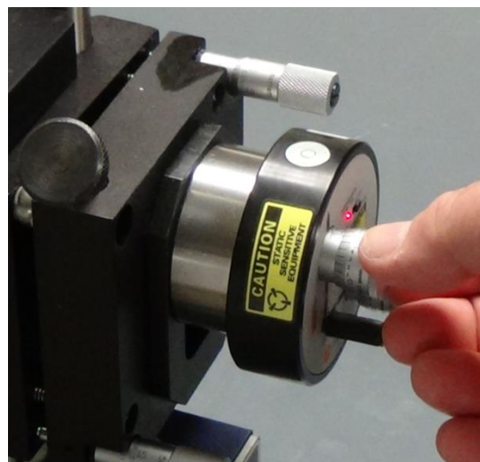
Fine adjust – uses the L-706 Micrometers.
