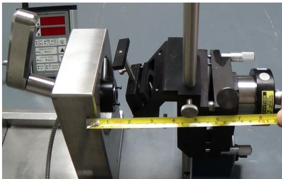
Figure 32-- D1 Distance Measurement: Center L-111 posts to mid-point of the target in Near Bore
