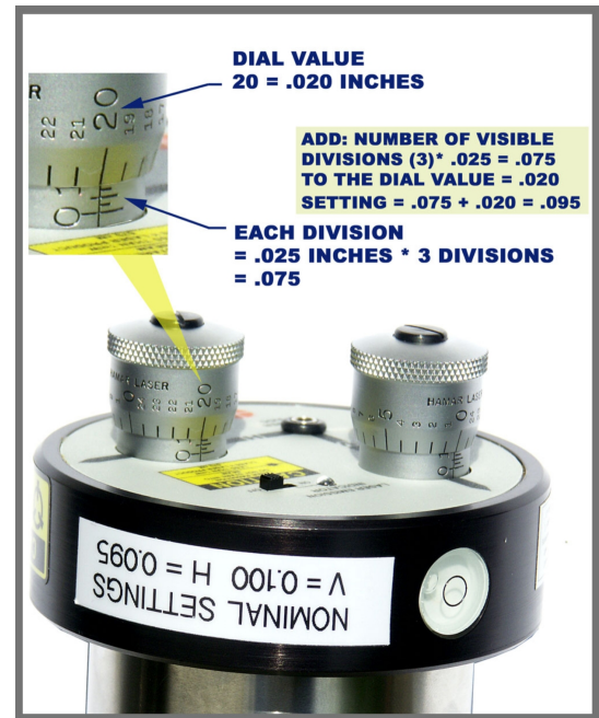
Figure 2 – Laser Micrometer Adjustments
