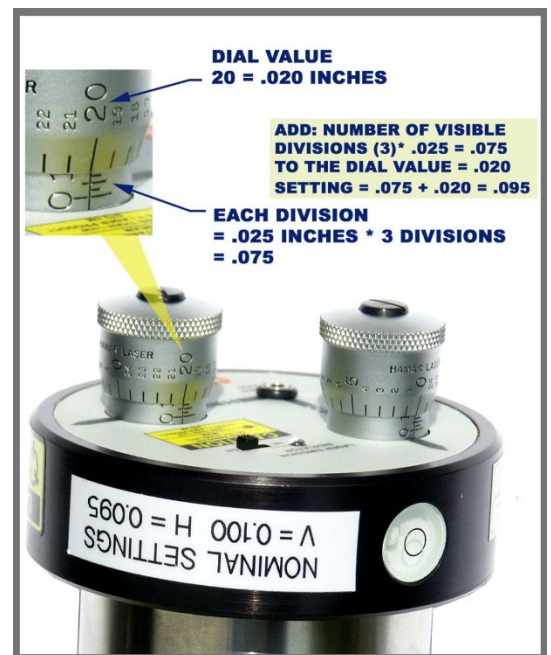
Figure 2 - Adjusting L-706 Micrometers
