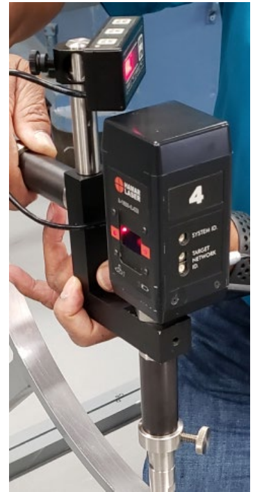
Figure 11 - R-1308 Mounted on A-1511 Wand Bore Fixture
