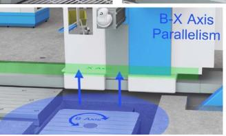
3. Again, rotate the table 90 degrees. The target now reads .0043, which is higher than the previous point and means the rotation plane is also sloping up and away from the spindle relative to the main table.
