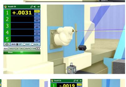
To compare to the X-Axis, start at 90 degrees and zero the PDA. Rotate to 270 degrees. The -.0019 reading indicates that the spindle axis is pointing to the left relative to the X-Axis.
