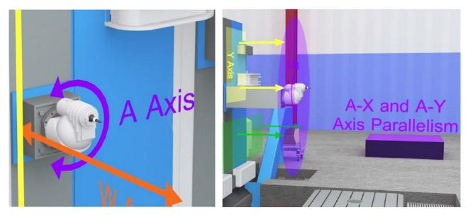
1. To measure the A rotation, we'll use the gold laser plane and a target mounted on the spindle. For both the A-Axis and the Tram measurements, a simple tram bar can be inserted into the spindle with a target attached.
