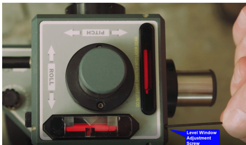
Figure 14 – L-733 (top view) showing location of Precision Level Vials and corresponding adjustment screws. Also see our YouTube video: How to Calibrate Level Vials .
