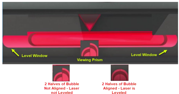
Figure 10 –L-740SP Split-Prism Level Vial Assembly for L-740 Series Lasers
